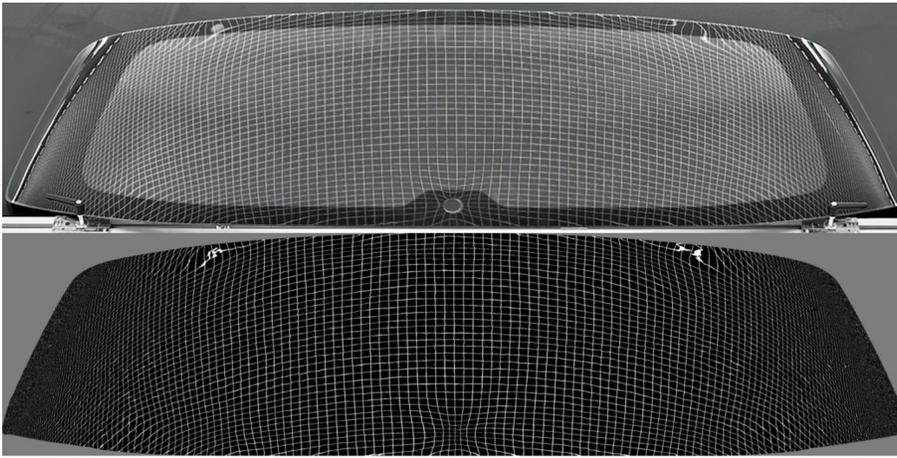
Reflective Output Report Comparing a Simulated Grid Board to an Actual Photograph
